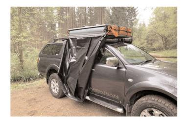
Slide the ladder out and whilst pulling down on the end of the ladder, walk backwards away from the vehicle, allowing the tent to unfold.
