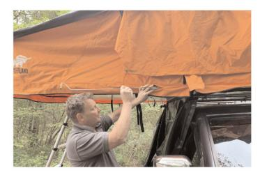
Flex support rod to engage hook end with the eyelet in the corner of the fly.
