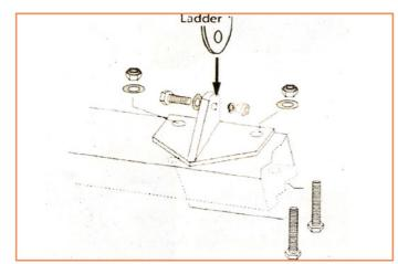
Attach the ladder to the brackets using the bolts. flat washers. and nuts, placing plastic spacers between the ladder mounts and brackets.
