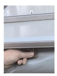
Slide 2 mounting nuts into the mounting rails and align with the holes. Locate the mounting holes under the mattress and insert the 40mm bolts and flat washers from inside out. Tighten the nuts and bolts firmly to attach the mounting rails to the tent floor
